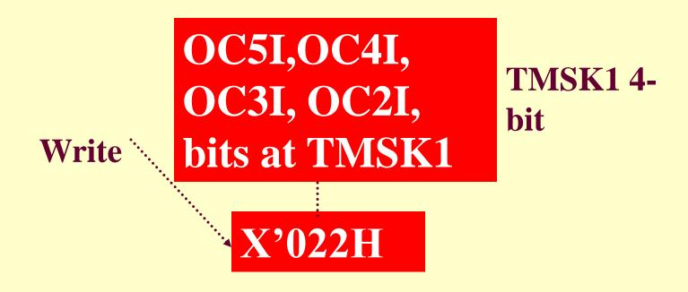
By a write OL-OM operation, define the level (1) and mask output pin action are defined for timer reading out compare output action (s) on selected pin(s) between OC2 to IC5
