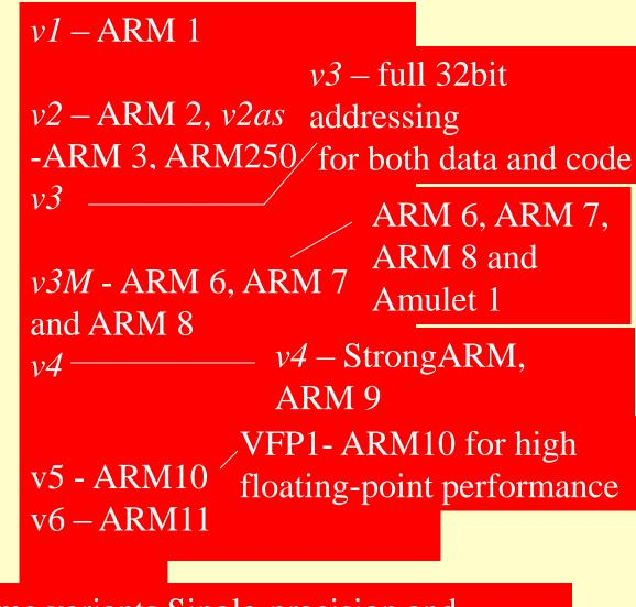
Some variants Single-precision and double-precision floating point arithmetic) on typical graphics and DSP algorithms
