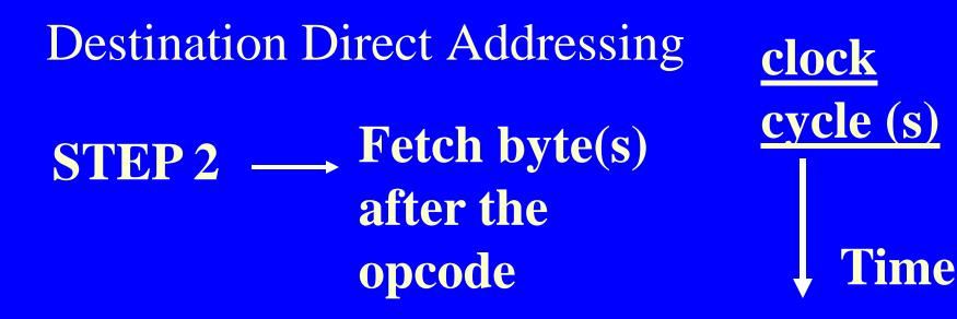
Addressing mode specifies that fetch byte(s) (next to the opcode of 8 bits) specify an address, destination operand is at that address.
