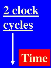
MOVX @Ri, A X specifies external memory, byte at Ri points indirectly to the address for the operand
