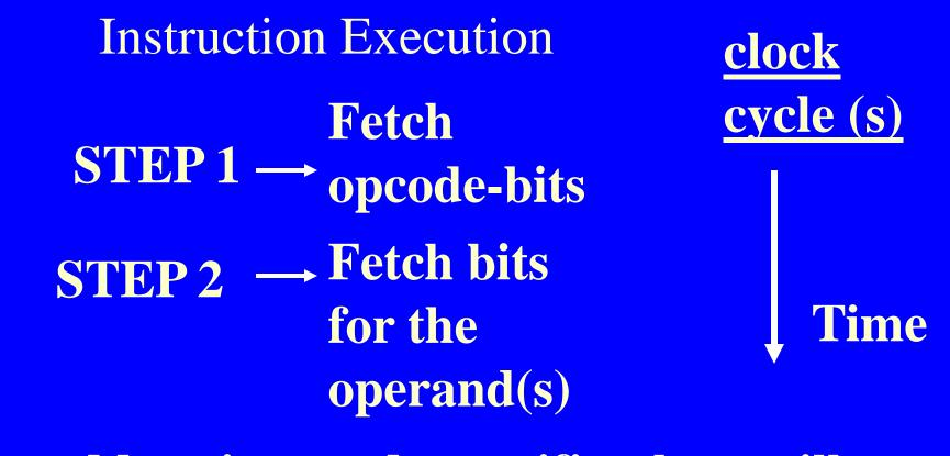
An addressing mode specifies, how will an operand(s) is obtained from the fetched bits before performing the operation(s) using it. Microcontrollers-... 2nd Ed. Raj Kamal 2011 4
