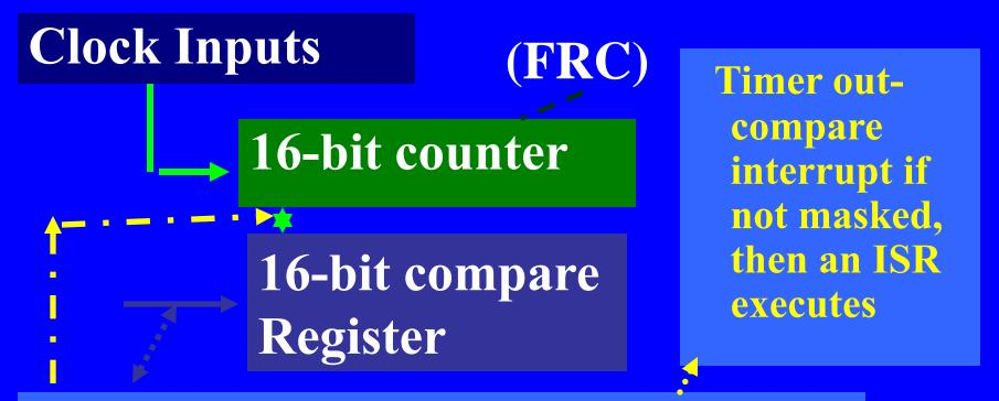
Compare both registers, on equality force an output level 0 or 1 or toggle output if comparison enabled
