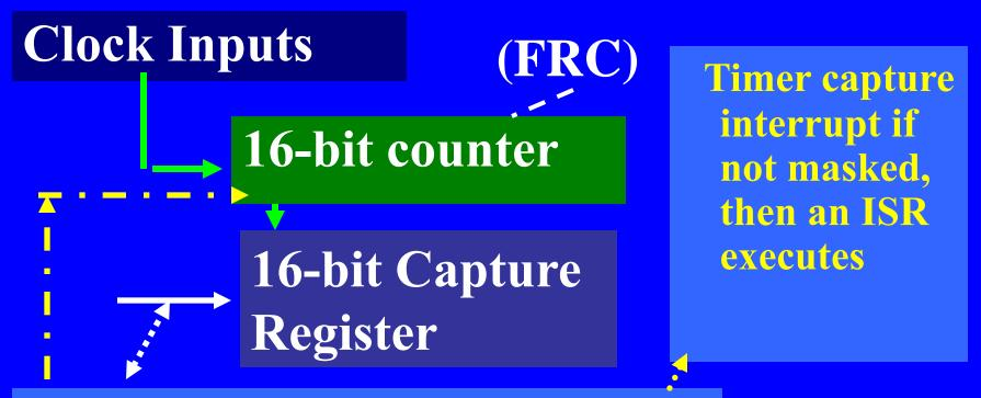
An edge forcing copying of the counter reading x into Capture Register if capture enabled
