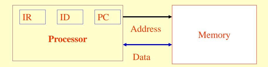
• Decode it to determine what the instruction is in Step 2) Processor decodes instruction and places at ID register
