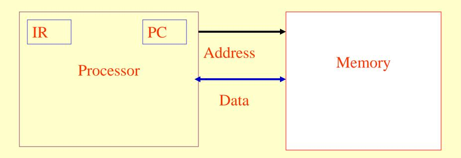
• Fetch an instruction from memory: Steps 1a and 1b) Processor requests instruction from memory using address in PC (or IP) register
