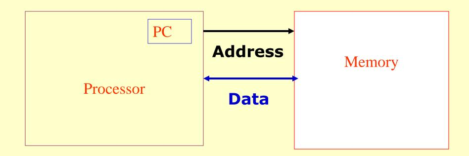
• Write the result back into the registers at the register file and PC updates Steps 5a and 5b) Result of instruction written back for register or memory and PC updates for next instruction
