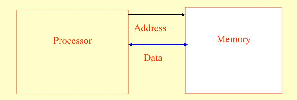
Step 1) Processor requests instruction from memory using address in Program Counter PC register
