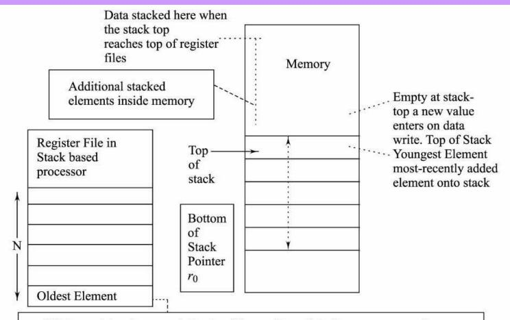
SP at a register always pointing to address of top of stack—moves up or down as amount of data in the stack pushes first at register file then into memory.
