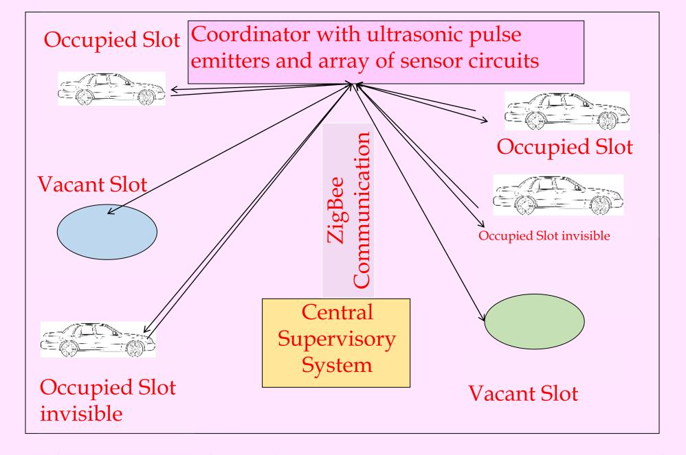
Fig. 12.11 Principle of designing the set up for identifying vacant spaces using ultrasonic pulses and back reflections from cars to the transceiver at the coordinator
