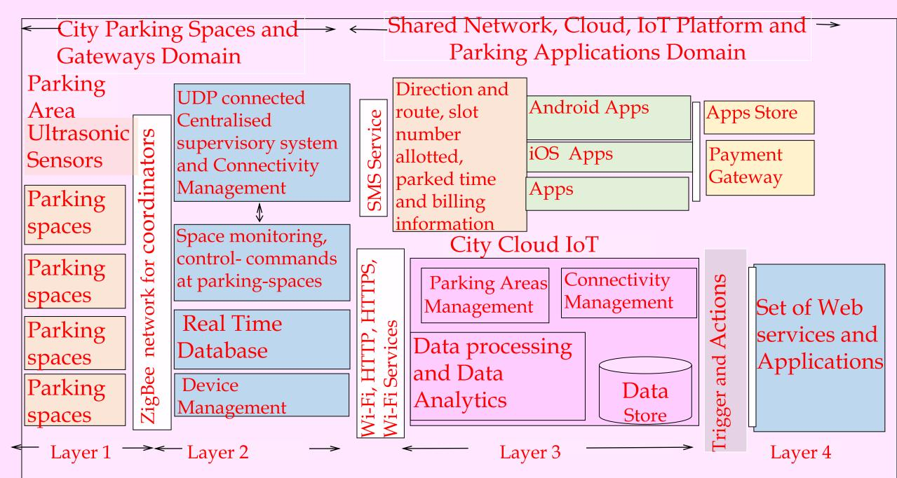
Fig. 12.10 Data flow diagram, domain-architecture reference-model for the smart parking applications and services
