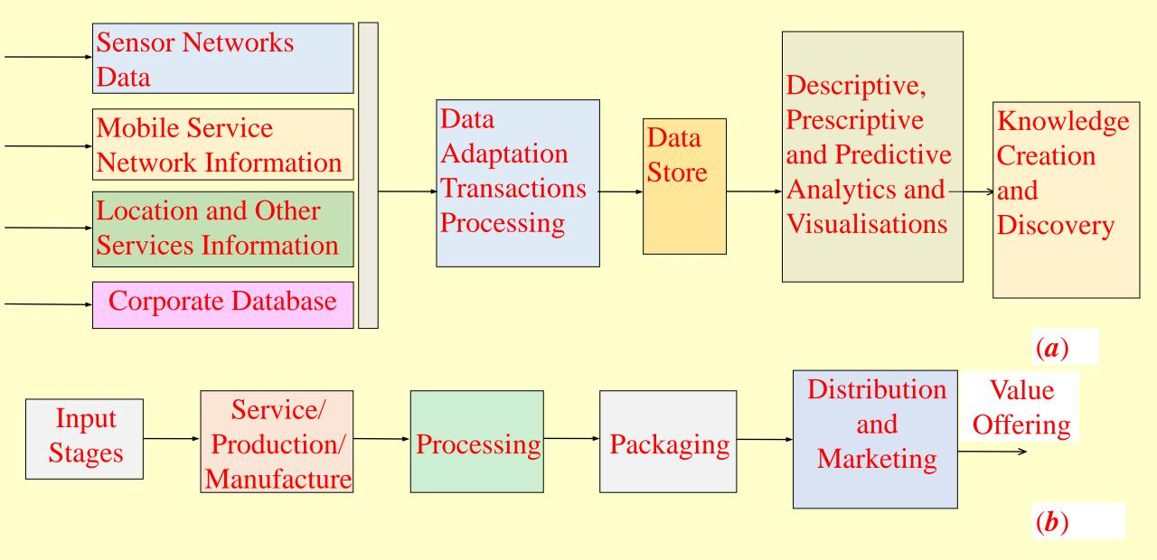
Fig. 11.5(a) and (b): Value creation using information driven IoT value chain and using production/manufacture driven value chain 10: "Internet of Things", Raj Kamal, Publs.: McGraw-Hill Education
