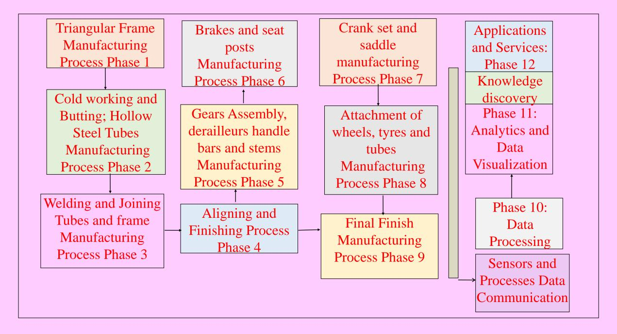
Fig. 7.10 IIoT phases in bicycle manufacturing process
