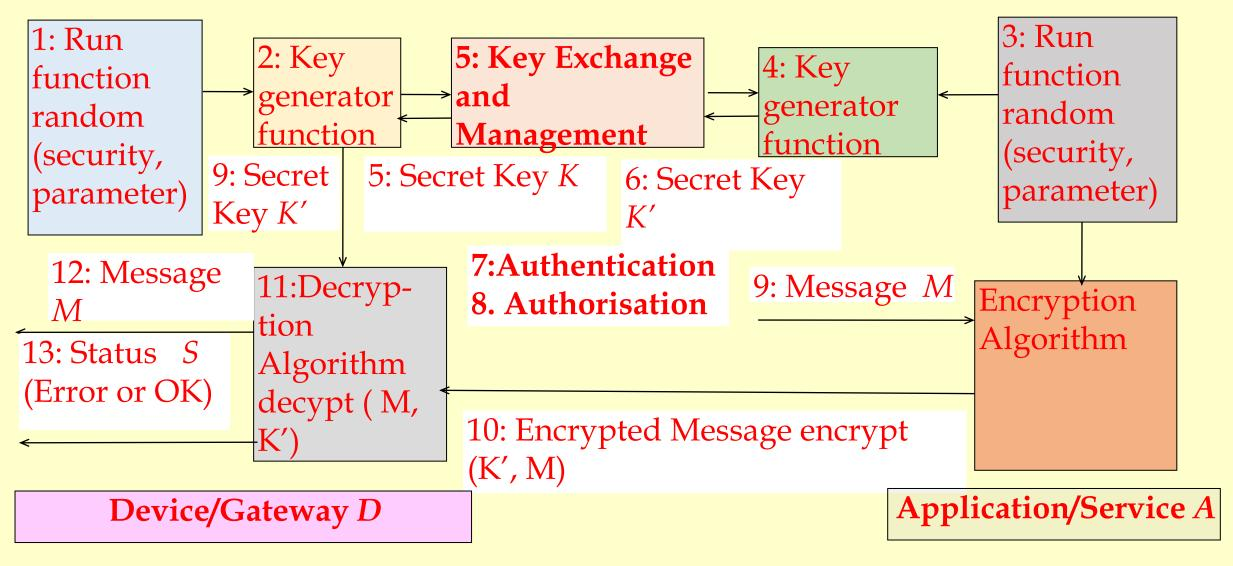
Fig. 10.5 Steps during Key exchanges and management, Authentication and authorizations followed by secure communication of Application/Service Message to the Device/Gateway
