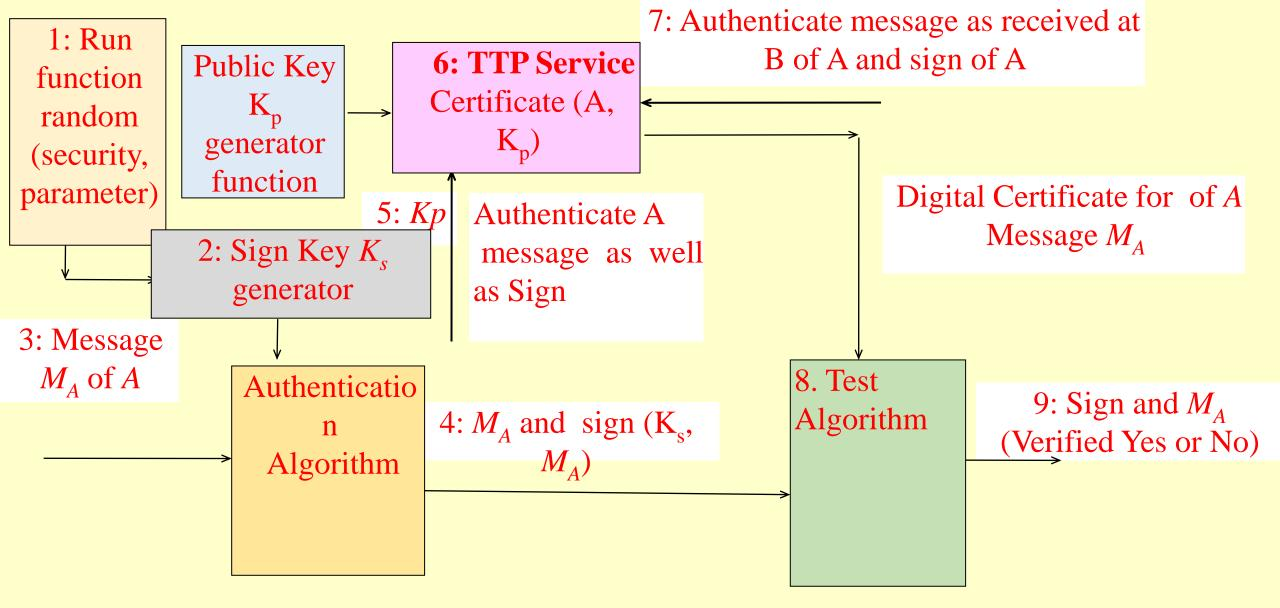
Fig. 10.6 Use of TTP Service and steps for signing, issue of digital certificates to a signed message and verification of signed message
