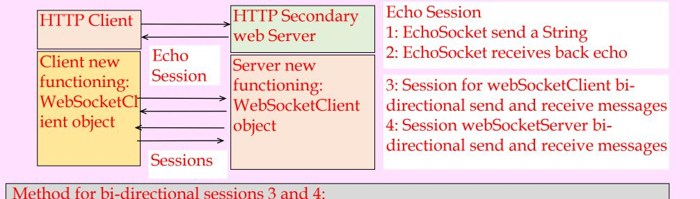
Fig. 9.6 Sequences of Sessions for message exchanges when using the webSockets
