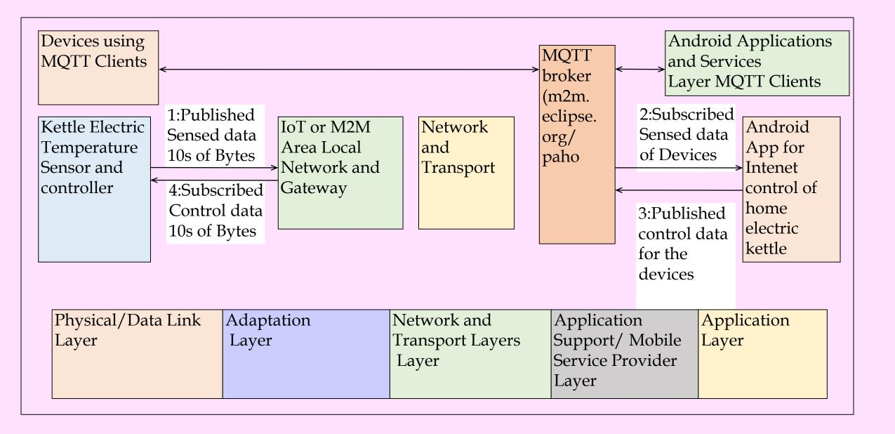
Fig. 9.3 Connected Sensor and Actuator publishing the sensed data and subscribing for the control data using MQTT Android clients' communication with Application layer MQTT clients through an MQTT Broker
