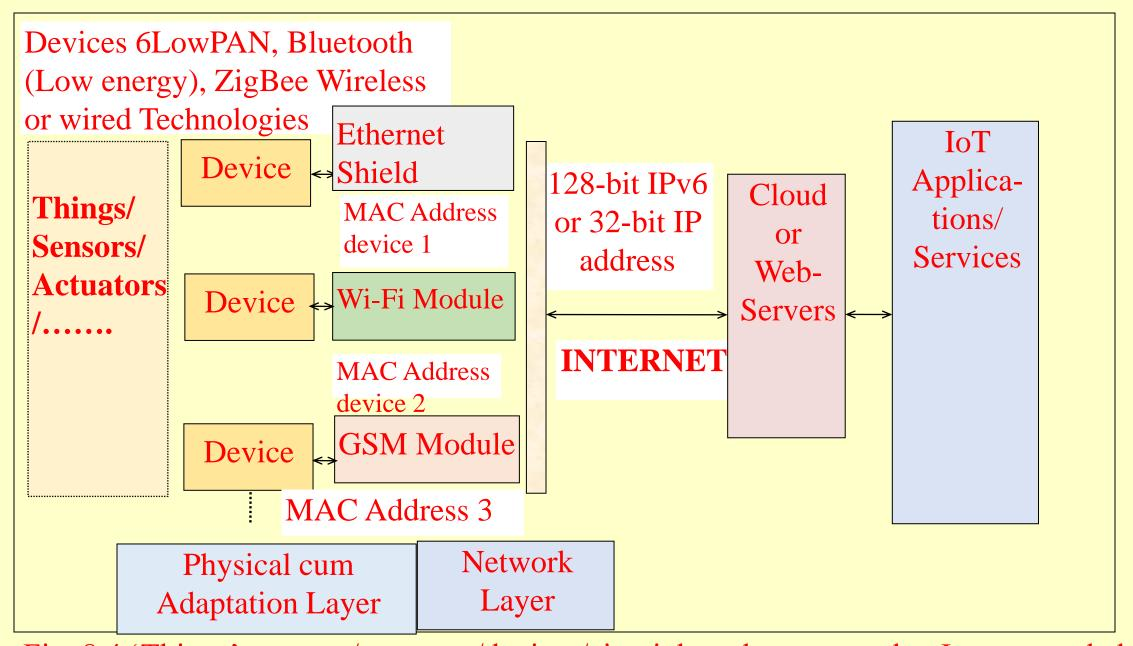
Fig. 8.4 'Things', sensors/actuators/devices/circuit boards connected to Internet and cloud or web-Servers for Applications and Services
