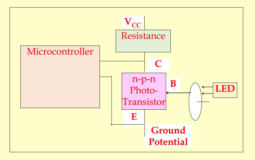
**Fig. 7.5** Microcontroller electronic circuit for a rotating wheel, rotation-completion sensing which senses two states (completion or incomplete) and generate two outputs 1 or 0 for the port pin
