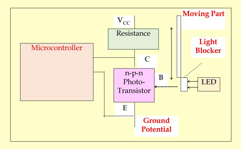
**Fig. 7.6** Microcontroller electronic circuits for sensing that a moving part reaching at a specific location and sensing two states (reached or yet to reach) and generate two outputs 1 or 0 for the port pin
