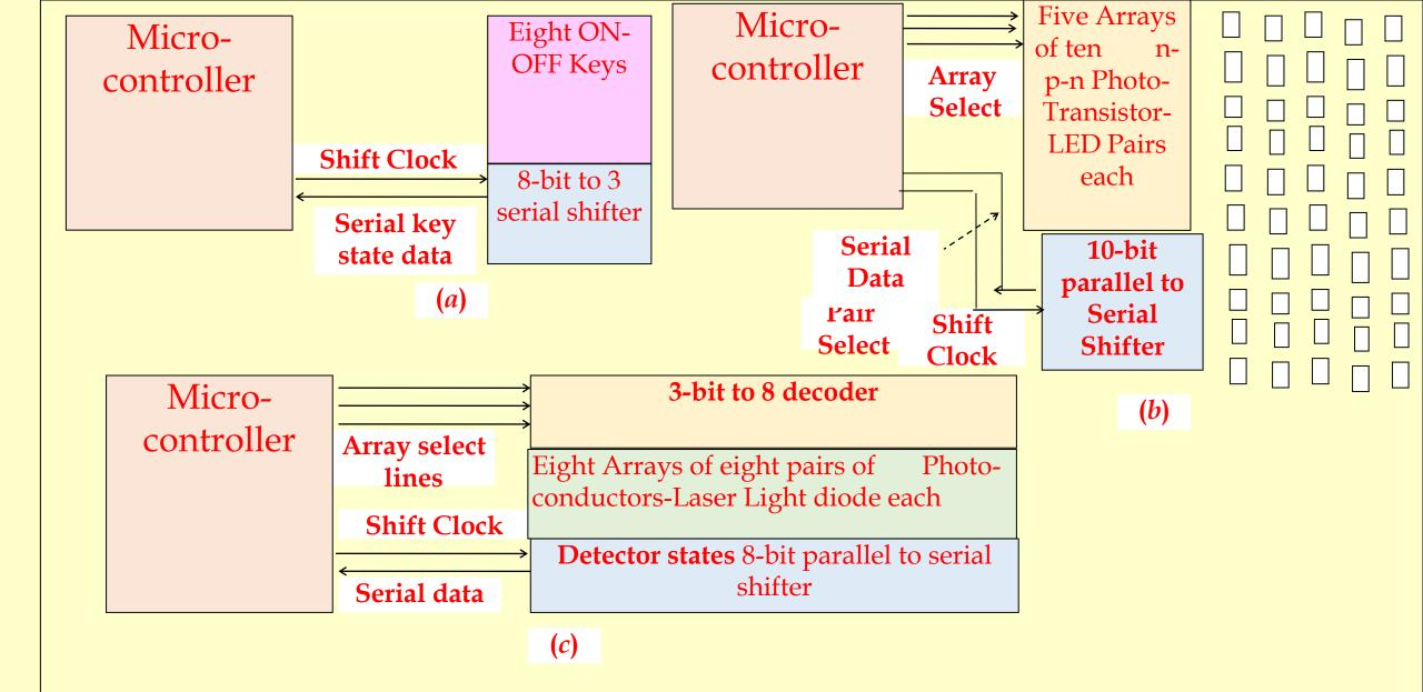
**Figs. 7.7**) Microcontroller electronic circuits for sensing ON-OFF states, five arraya of 10- light passing slots each for detecting sales level for five types and ten levels of sales of each type, and (c) array of 64 parking slot sensors
