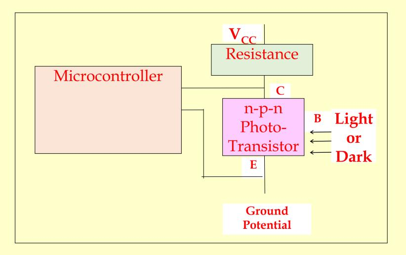
**Fig. 7.4** Microcontroller electronic circuit for a streetlight environment ambient condition sensor witch senses two states and generates two outputs 1 or 0 for the port pin
