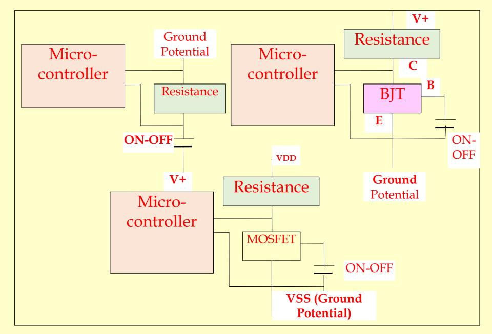
Fig. 7.3 Circuits for sensing ON and OFF key states; Generation of 1 and 0 for the port pin
