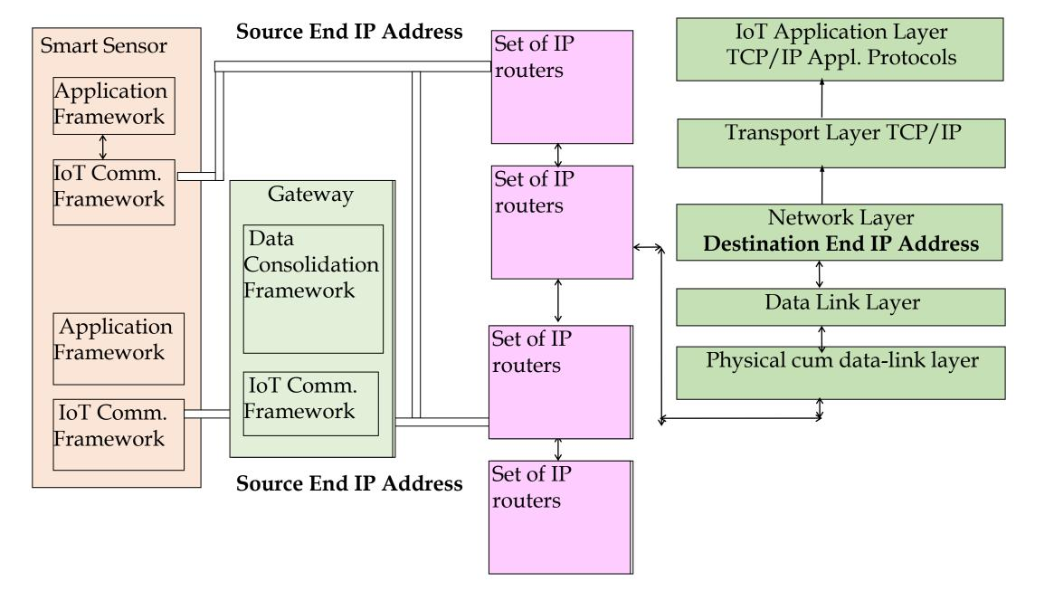
Fig. 4.1 Source end network layer connected through set of IP routers for data packets from an IP address and communicating with IoT/M2M IoT Apps and Services layer using TCP/IP suite of Application protocols
