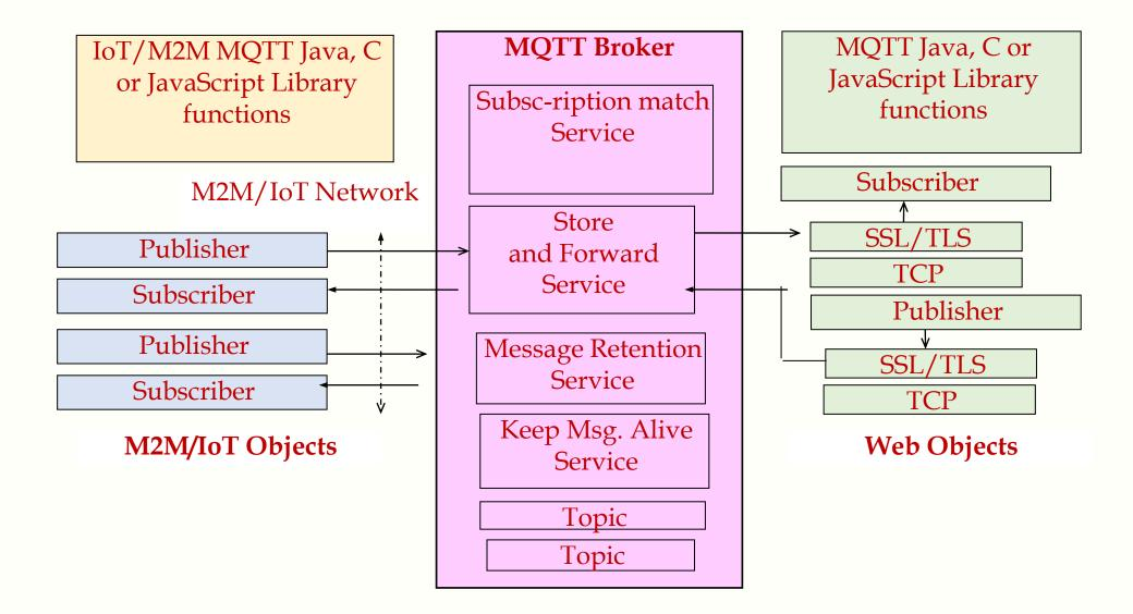
Fig. 3.6 M2M/IoT device objects (publisher and subscriber) messaging to web objects (publisher and subscriber) using an MQTT Broker.
