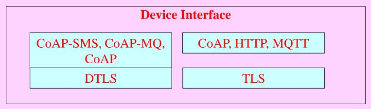
**Fig. 1.7** mbed<sup>™</sup> API and device interfacing components
