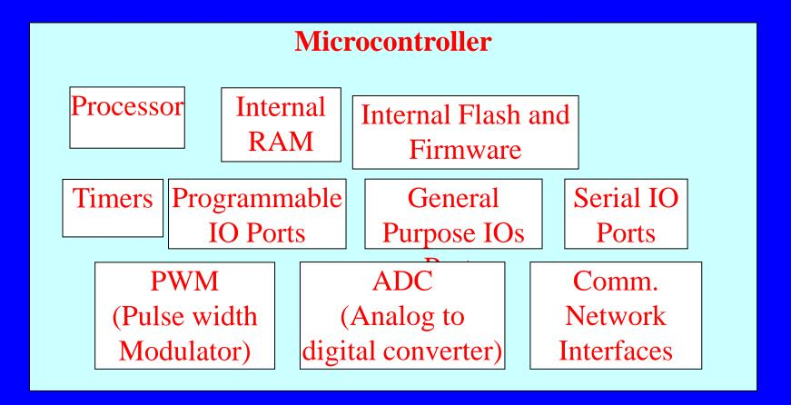
Fig. 1.6 Various functional units in a microcontroller embedded in IoT device
